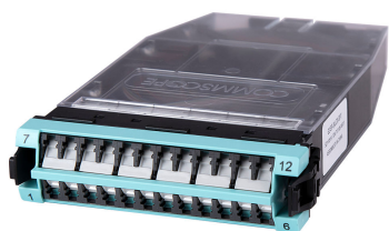
G2 Splice Cassette, 24LC with internal shutters, OM4, with ribbon pigtails
